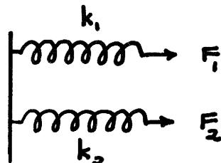
$$\text{Hence } k_{\text{eff}} = k_1 + k_2 \quad \text{and} \quad \omega_b = \sqrt{\frac{k_1 + k_2}{m}}$$
