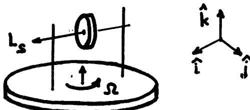
The spin angular momentum is  $L_s = I_o \omega_s$ . Assuming that the axle is close to horizontal,  $| \frac{dL}{dt} | = \Omega L_s$  along the  $\hat{j}$  axis.
