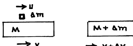
$$\text{Hence } M \frac{dv}{dt} + \frac{dM}{dt}(v - u) = 0 \quad \text{since } \frac{dm}{dt} = \frac{dM}{dt}$$
