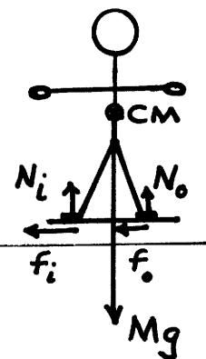
$$\text{Solving, } N_{\text{inside}} = \frac{1}{2} \left[ Mg - \frac{Mv^2 L}{R(d/2)} \right]$$
