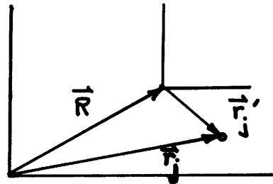
$$\begin{aligned}\vec{L}' &= \sum \vec{r}'_j \times \vec{p}'_j = \sum (\vec{r}_j - \vec{R}) \times \vec{p}'_j \\ &= \sum \vec{r}_j \times \vec{p}'_j - \vec{R} \times \sum \vec{p}'_j = \vec{L} \quad \text{since } \sum \vec{p}'_j = 0\end{aligned}$$
