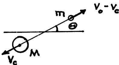
$$v_f^2 = v_c^2 + (v_0 - v_c)^2 - 2v_c(v_0 - v_c) \cos(\pi - \Theta)$$
