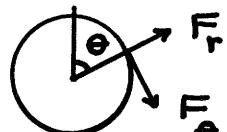
$$F_\theta / \left. \frac{GM_e m}{r^2} \right|_{45^\circ} = (5.4 \times 10^{-4})(6) \frac{1}{\sqrt{2}} \frac{1}{\sqrt{2}} = 1.62 \times 10^{-3}$$
