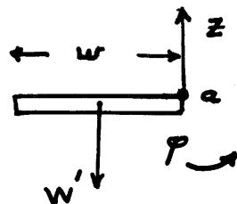
Consider the motion of the truck door in a system fixed to the truck. The door appears to "fall" from rest in a gravitational field  $g' = A$ .
