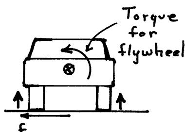
In the absence of the flywheel, the counterclockwise torque due to the normal forces at the wheels must oppose the clockwise torque due to the radial (transverse) friction force,  $f = Mv^2/r$ . With the flywheel, the normal forces exert no torque; so the flywheel must exert a clockwise torque  $= Lf$ , where  $L$  is the distance from the road to the center of mass. The counterclockwise torque  $Lf$  must be just sufficient to make the flywheel precess at the rate the car is turning.
