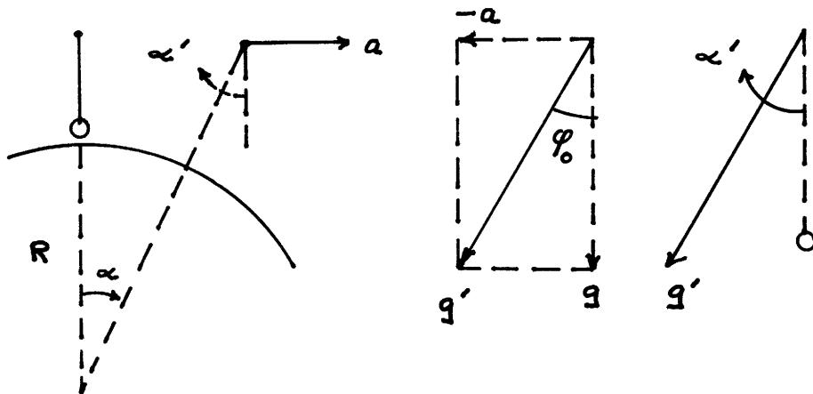
For the pendulum to point continually toward the earth, its angular acceleration  $\alpha'$  must be equal and opposite to the angular acceleration of its point of support with respect to the center of the earth,  $\alpha = \frac{a}{R}$ .
