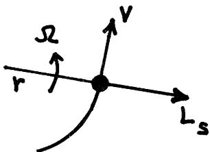
The torque due to the road is  $\tau = Lf = Mv^2 RL$
