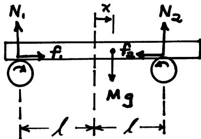
$$\text{Horizontal Force} = f_2 - f_1 = \mu(N_1 - N_2) = -\frac{\mu Mg}{l} x$$
