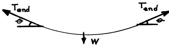
$$(b) T_{\text{middle}} = T_{\text{end}} \cos \theta = \frac{W}{2 \tan \theta}$$
