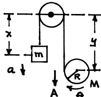
**6.24** Both drums turn through the same angle and therefore have the same angular acceleration. (The torques about the centers are identical)
