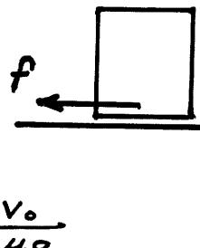
$$\text{Glass comes to rest at } t_0 = \frac{v_0}{\mu g}$$
