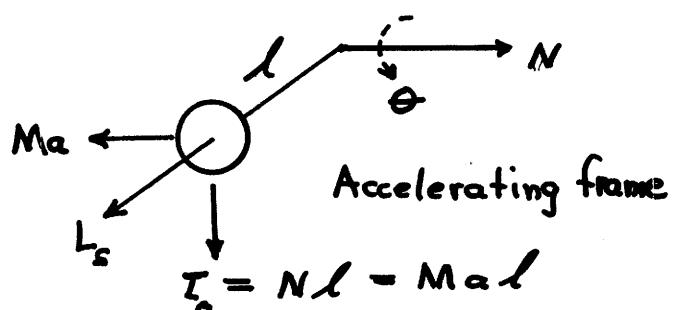
In the accelerating system, gyroscope sees an effective gravitational field  $-\vec{\alpha}$  and precesses under the torque
