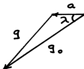
The apparent acceleration of gravity is  $\vec{g} = \vec{g}_0 - \vec{a}$ , where  $\vec{a}$  is the acceleration of the local reference frame.
