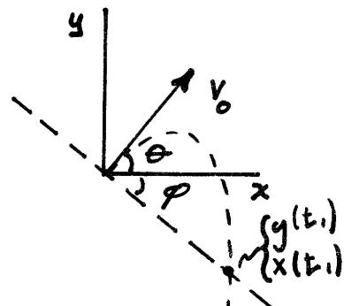
$$t_1 = \frac{x(t_1)}{v_0 \cos \theta}$$
