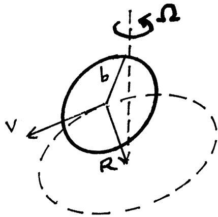
Coin is accelerating, so we must use CM as origin for torque equations.
