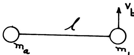
$$\dot{R} = \frac{m_a v_a(0) + m_b v_b(0)}{m_a + m_b} = \left( \frac{m_b}{m_a + m_b} \right) v_0$$
