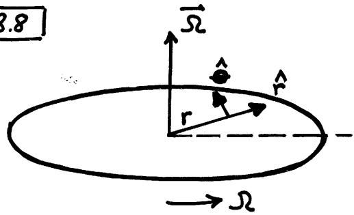
$$\vec{v}_{\text{inertial}} = \vec{v}_{\text{rot}} + \vec{\Omega} \times \vec{r}$$
