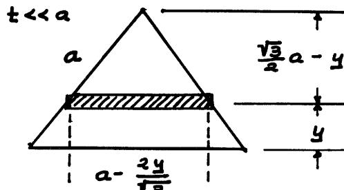
$$y = \frac{4M}{M\sqrt{3}a^2t} \int_0^{\frac{\sqrt{3}}{2}a} \left(a - \frac{2y}{\sqrt{3}}\right) y dy t = \frac{a}{2\sqrt{3}} = \frac{1}{3} \frac{\sqrt{3}a}{2}$$
