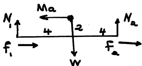
$N_1, N_2$  are the normal forces on the wheels,  $f_1$  and  $f_2$  are the frictional forces, and  $Ma$  is the fictitious force.
