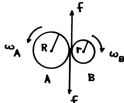
$f$  continues to act until the surfaces of contact attain the same linear velocity:  $R\omega_{A,f,in} = r\omega_{B,f,in}$ .
