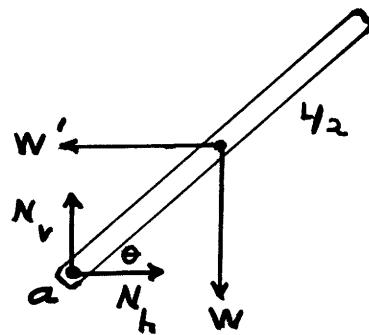
The force diagram is in the accelerating system.  $\vec{W}'$  is the fictitious force:  $\vec{W}' = -M\vec{A}$ . The torque about the pivot point is
