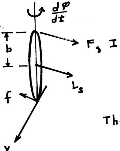
During the blow, the forces acting are the impulsive force  $F$  and the frictional force  $f$ . We assume  $F \gg f$  and neglect  $f$ .
