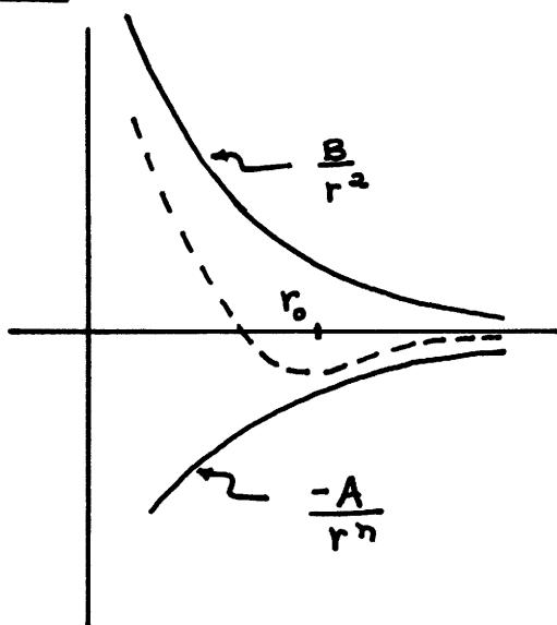
$$\begin{aligned}U_{\text{eff}} &= u + \frac{\ell^2}{2\mu r^2} \\&= -\frac{A}{r^n} + \frac{B}{r^2}, \quad B = \frac{\ell^2}{2\mu}\end{aligned}$$
