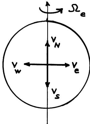
(a) East :  $\vec{\Omega} \times \vec{v}$  points radially out
