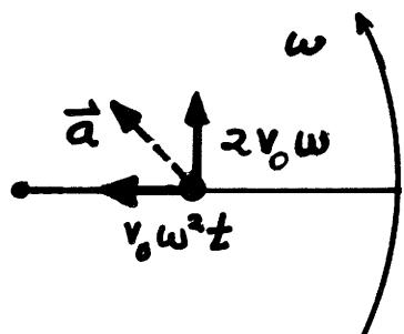
$$\text{Hence } \vec{a} = -v_0 \omega^2 t \hat{r} + 2v_0 \omega \hat{\theta}$$
