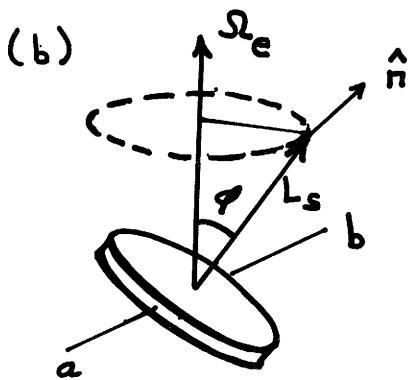
Let the gyro spin axis be at angle  $\varphi$  with respect to  $\Omega_e$ . The rate of change of spin angular momentum in the direction  $\hat{n}$  is  $L_s \sin \varphi \Omega_e \approx L_s \varphi \Omega_e$
