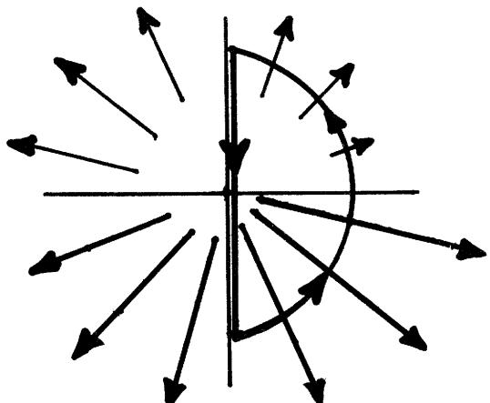
The work around the indicated closed path is zero over the curved part but not zero over the straight part, because  $\vec{F}$  has a different magnitude at  $90^\circ$  and  $180^\circ$ .
