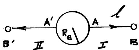
Suppose the ground station sends a signal to the satellite at time  $T_I$ , in position I, and at time  $T_{II}$ , twelve hours later, in position II.
