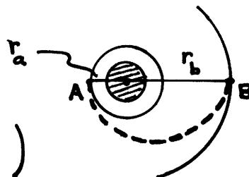
$$E' = -WR_e \left( \frac{1}{\frac{r_a}{R_e} + \frac{r_b}{R_e}} \right) = -WR_e \left( \frac{1}{2+4} \right) = -\frac{1}{6} WR_e$$
