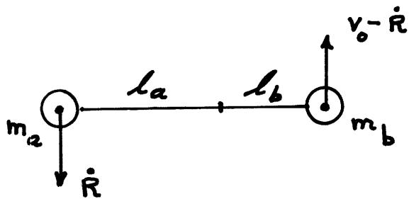
$$\omega = \left( \frac{m_b v_0}{m_a + m_b} \right) / l_a = \frac{v_0}{l}$$
