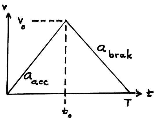
$$v_0 = a_{acc} t_0 = a_{brak} (T - t_0)$$
