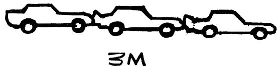
Hence  $\frac{1}{2}E_i - \frac{1}{6}E_i = \frac{1}{3}E_i$  is dissipated in the second collision, divided between C and the other cars.
