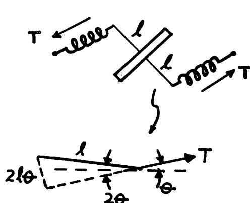
The torque due to each spring is  $2l\theta T$ .
