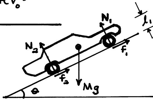
$$\begin{aligned} 0 &= N_1 l_2 - N_2 l_2 + f_1 l_1 + f_2 l_2 \\ &= (N_1 - N_2) l_2 + (Mg \sin \theta) l_1 \end{aligned}$$
