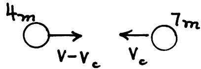
Energy in the C system is  $E_c = \frac{1}{2}(4m)(v - v_c)^2 + \frac{1}{2}(7m)v_c^2$
