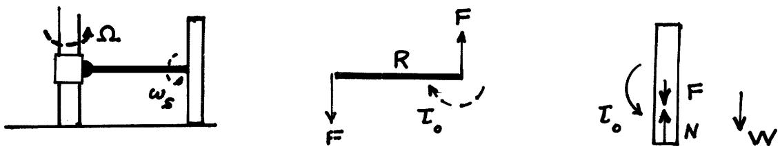
The axle exerts a torque  $T_0$  on the millstone and a vertical downward force  $F$ . The millstone exerts opposite force and torque on the axle. The coupling at the vertical column must also exert a downward force  $F$  on the axle.
